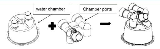
**Step2**: Fit the water chamber to the main unit by pressing down the finger guard on the High-flow Humidification Device and sliding the water chamber on. Push the water chamber on firmly until the finger guard clicks into place.
